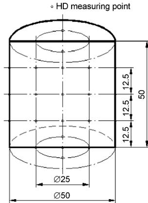
Fig. 4. Hardness measuring points.
