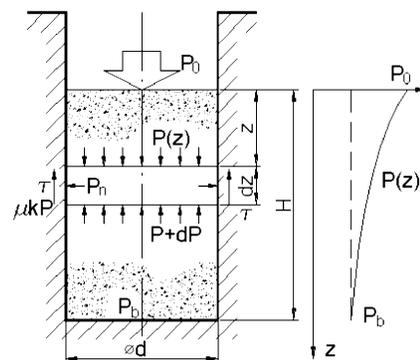
Fig. 2. Scheme of the compaction model.
