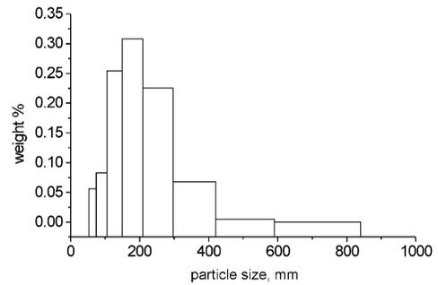
Fig. 3. Sieve analysis results of the silica sand used in this study.
