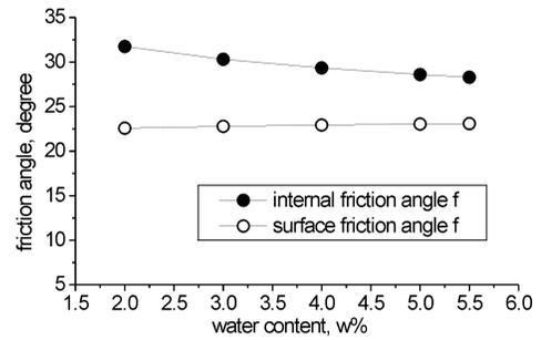
Fig. 11. Internal friction angle and surface friction angle ( $w\% = 3.0$ , Ben% = 10, SC% = 3).
