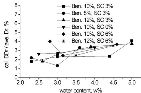
Fig. 14. Estimated relative density difference  $\Delta D_r$ .
