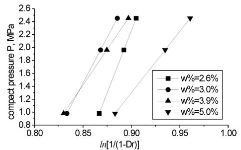
Fig. 7. Relative density vs. compaction pressure ( $P = 2.45$  MPa,  $Ben\% = 10, SC\% = 3$ ).
