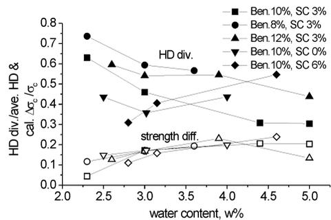
Fig. 12. The estimated  $\Delta\sigma_c$  compared with hardness difference at  $P = 0.98$  MPa.
