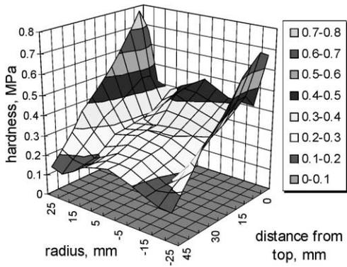
Fig. 9. Average hardness distribution on the central plane ( $P = 0.98$  MPa, Ben% = 10, SC% = 1,  $w\% = 3$ ).
