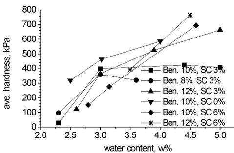
Fig. 10. Average hardness vs. water content ( $P = 2.48$  MPa).
