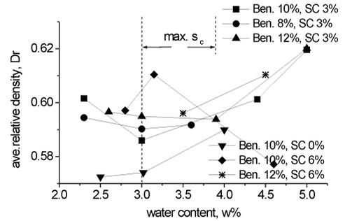
Fig. 6. Relative density vs. water content ( $P = 2.45$  MPa).
