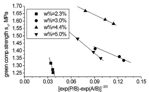
Fig. 8. Green compression strength vs. the factor derived from the S–M equation ( $P = 2.45$  MPa,  $Ben\% = 10, SC\% = 3$ ).
