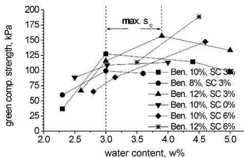
Fig. 5. Green compression strength of the green sands with different compositions ( $P = 2.48$  MPa).
