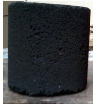
Fig. 1 Specimen of UFS prepared for compression strength.
