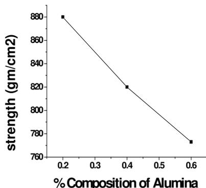
Fig. 4 Shows the Green compression strength of UFS.
