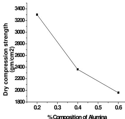
Fig. 5 Shows the Dry compression strength of UFS.
